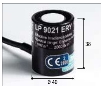
LP 9021 ERY: Radiometric probe for TOTAL EFFECTIVE IRRADIANCE ( W_{eff}/m^2 ) according to the UV action curve (CEI EN 60335-2-27) complete with SICRAM module. Spectral range: 250 nm...400 nm, quartz diffuser for cosine correction. Measurement range: 0.1 \cdot 10^{-3} W_{eff}/m^2 \dots 2000 W_{eff}/m^2 .
