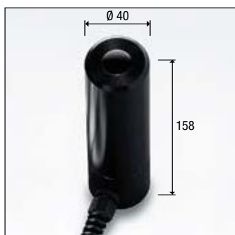
LP 9021 LUM6: Probe for measuring LUMINANCE , measuring range from 1 to 1999 x 10 3 candles/ m 2 . Measuring angle 2°. CIE filter for correction of the response according to the human eye, CIE n°69-UNI11142
